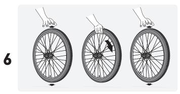
Bounce: Hold the wheel vertically and gently bounce or "dribble" it to disperse sealant throughout the inside of the tire. Let the wheel drop from an inch or two, then rotate a few degrees and repeat. Do this for several revolutions of the wheel.
