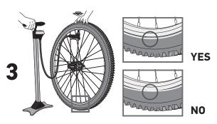
Rotate the valve to 12 o'clock, and install a pump. Inflate tire to 35psi (2.4 bar) to seat tire.
