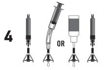
Add sealant: Once successful with inflation, remove the valve core to add Stan's sealant. Add 2-4oz. of sealant.
